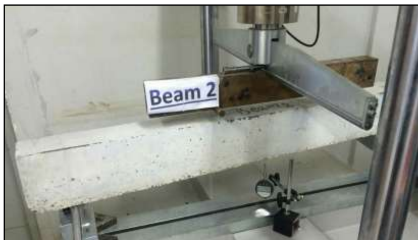
Plate 1. Set-Up of beam specimen test
