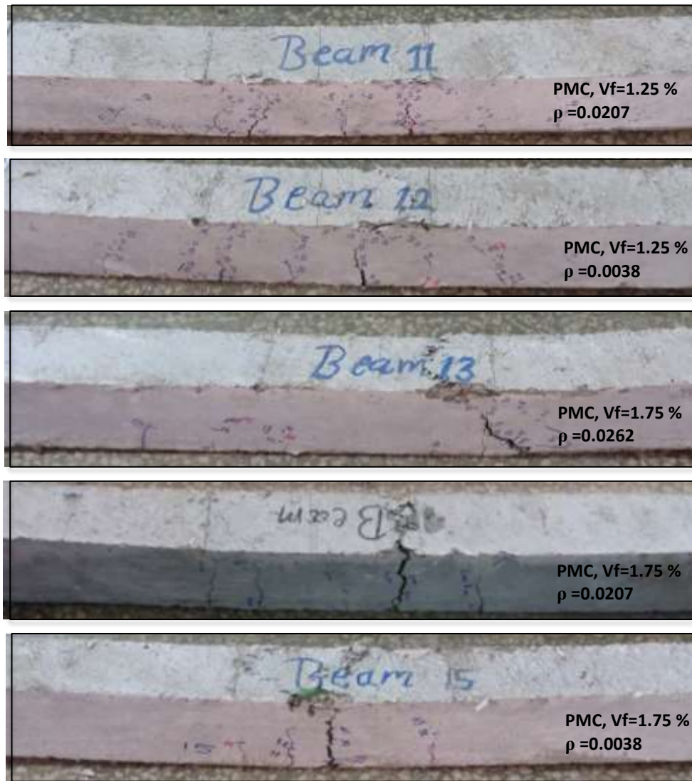
Plate 2. Failure mode of reinforced concrete beams made by polymer modified concrete with waste plastic fibre
