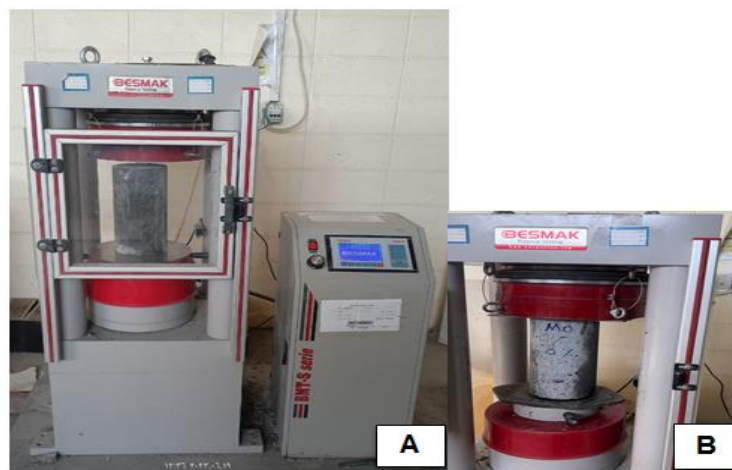
Fig 5. Compressive testing of specimens [A] The ELE-Digital testing compression machine, [B] The test sample.
