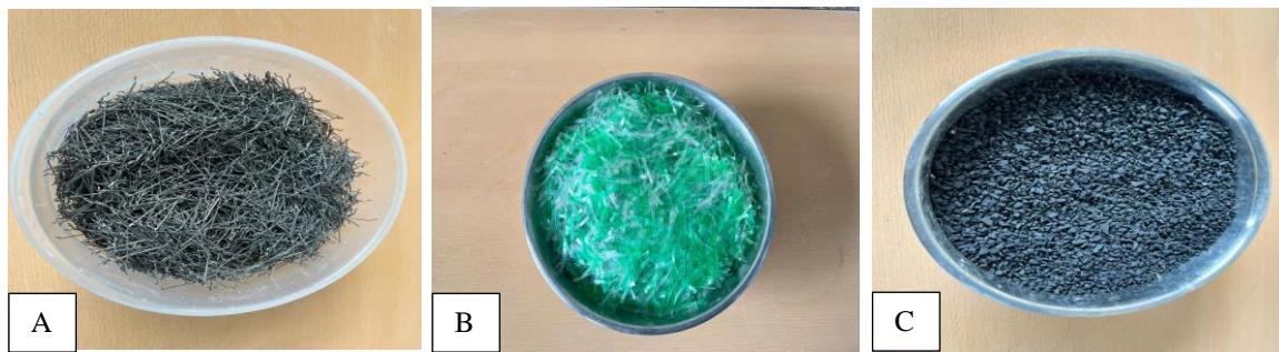
Fig. 2 Materials used in this study: (A) Steel fiber (B) PET fiber (C) Crumb rubber aggregate.
