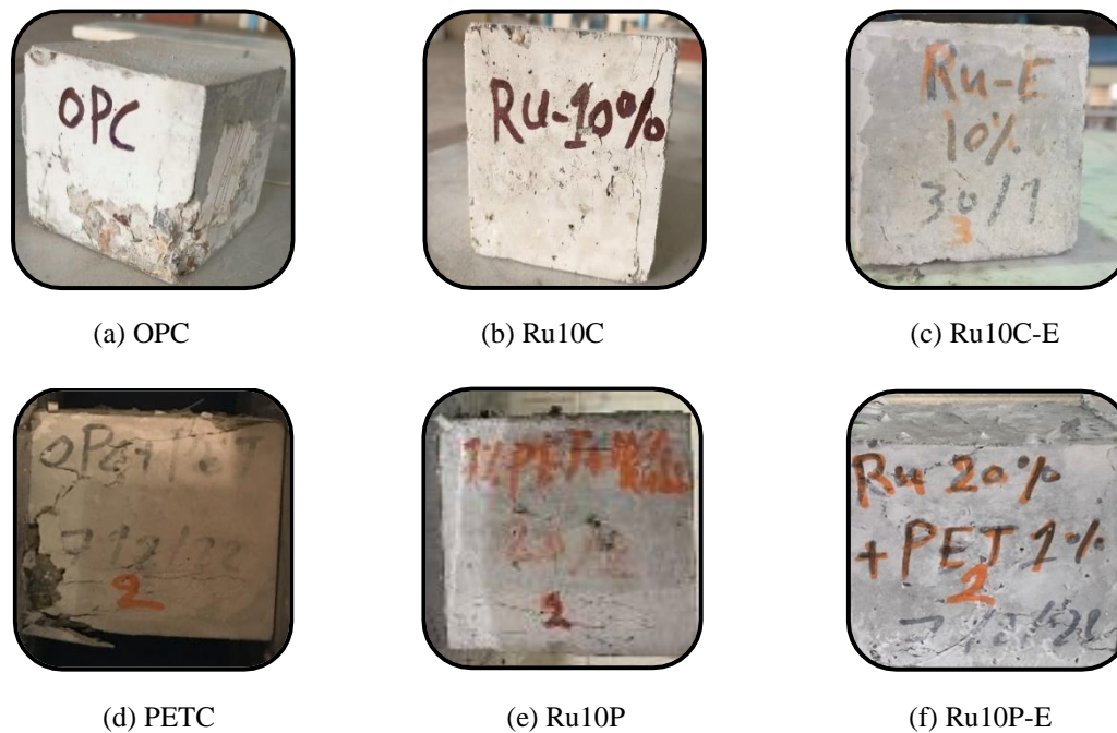
Fig. 5 Failure modes of concrete cubes
