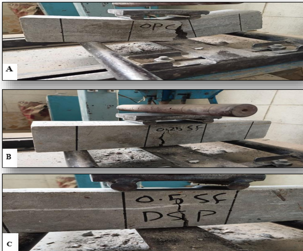
Fig.7 Failure mode of samples under flexural loads (A) plain concrete, (B) 0.25% DSF, and (C) 0.5% DSF.
