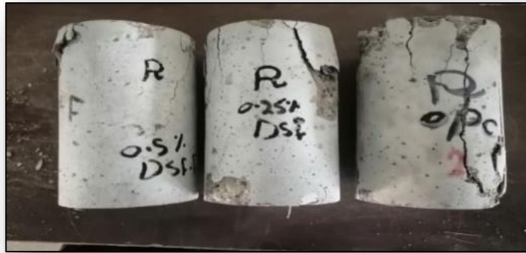
Fig.3 Failure mode of cylinders specimens.
