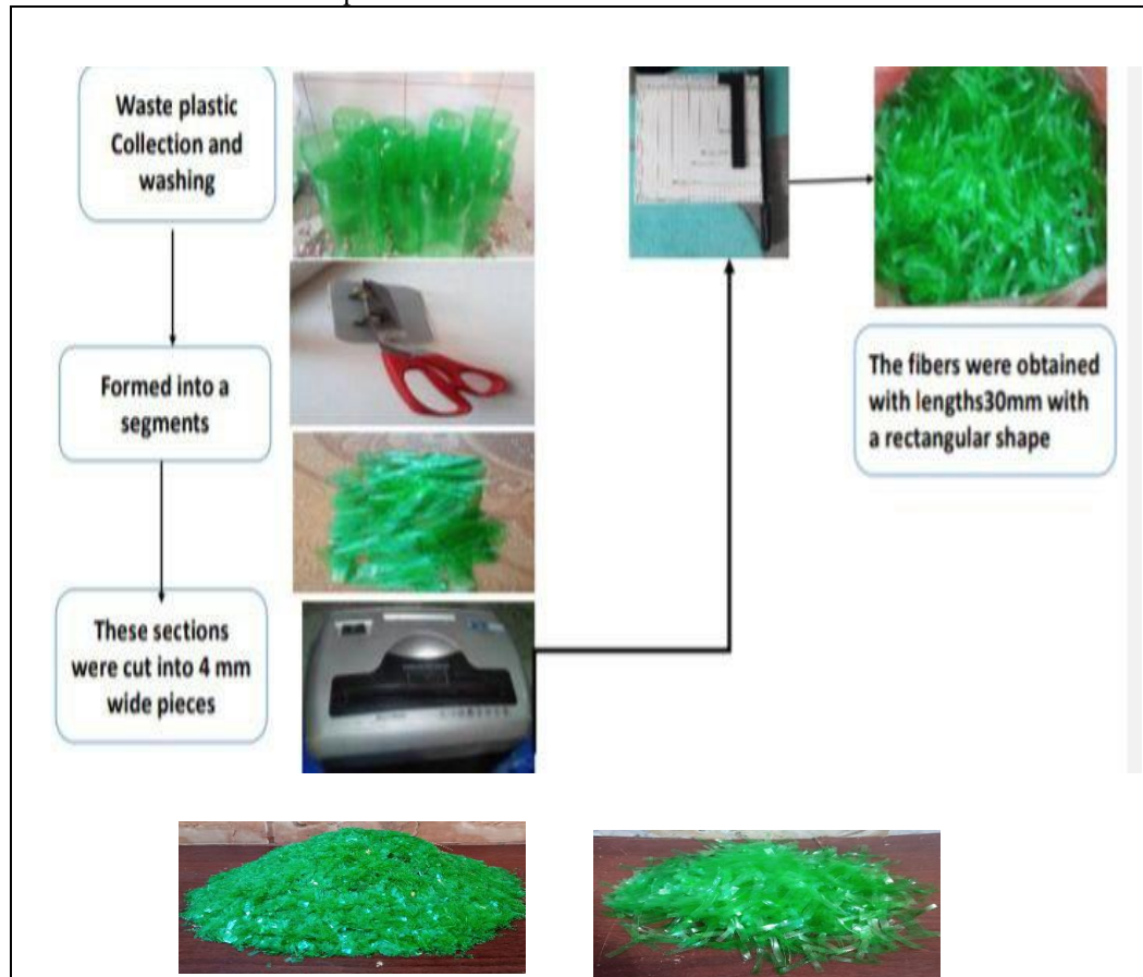
Fig .4 Method used to make PET fibers and PET fines
