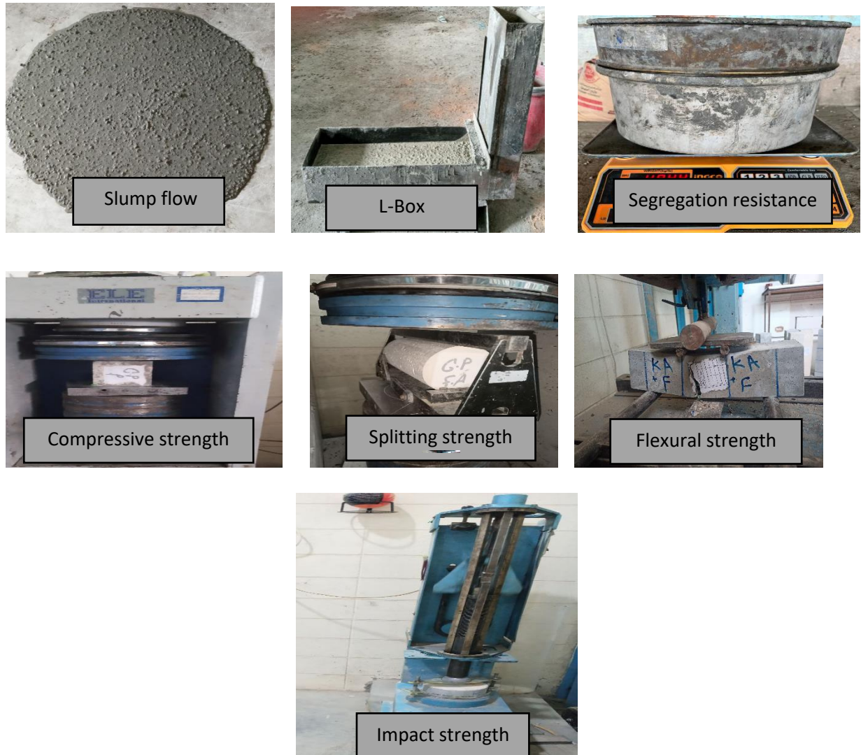
Fig .5 Tests of fresh and hardened properties of SCC
