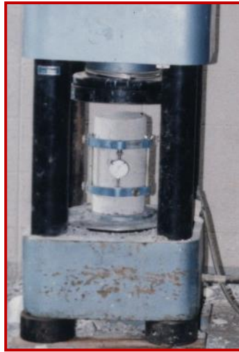
Fig. (1) Extensometer fixed to a cylindrical specimen during test for stress strain relationship
