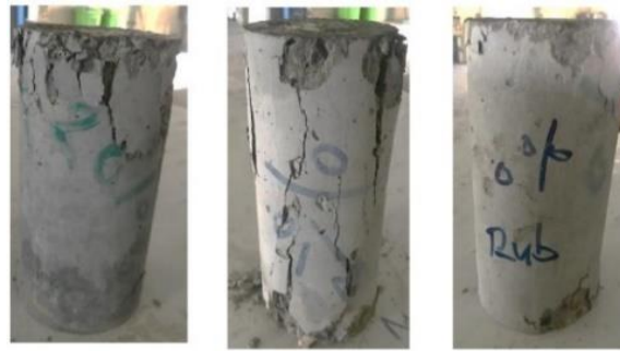
Fig.5 Failure mode of cylinders specimens.
