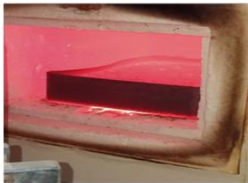
Fig. 1 Burning of the wastes in the oven at 900\text{ C}^\circ .
