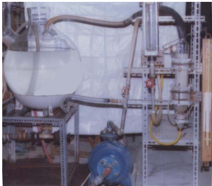
Fig. 3. Photographic picture of water flow through packed bed.
