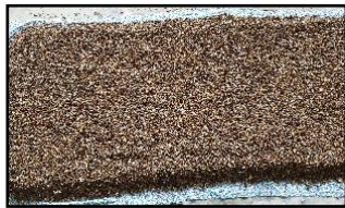
c) Coarse aggregate ( 980 \text{ Kg/m}^3 ) with maximum size 10 mm, and specific gravity 2.6
