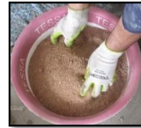
b) Fine aggregate ( 730 \text{ Kg/m}^3 ) with maximum size 4.75 mm and specific gravity 2.54
