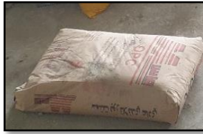
a) Portland cement ( 395 \text{ Kg/m}^3 ), and the water cement ratio (0.46)
