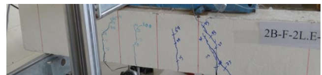
Figure 19 Cracks patterns of beam 2B-F-2L.E-90
