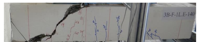
Figure 20 Cracks pattern of beam 3B-F-1L.E-140
