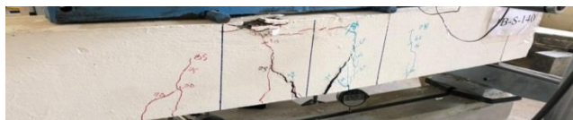
Figure 13 Cracks patterns of beam 1B-S-140
