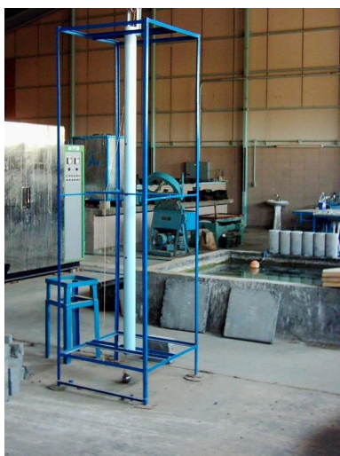
Plate (6) Low Velocity Impact Test Setup
