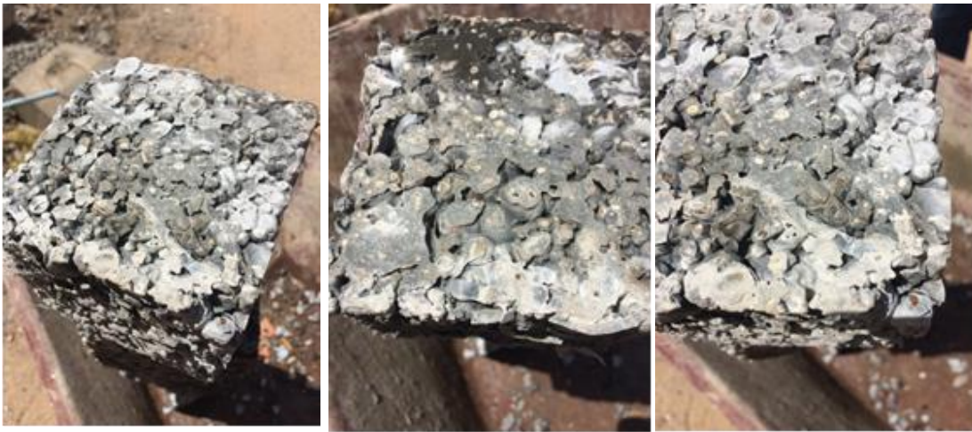
Figure 7. Mode of failure of samples containing WPFs and Polystyrene.
