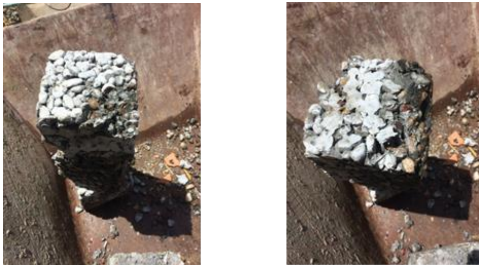
Figure 6. Mode of failure for reference mix.
