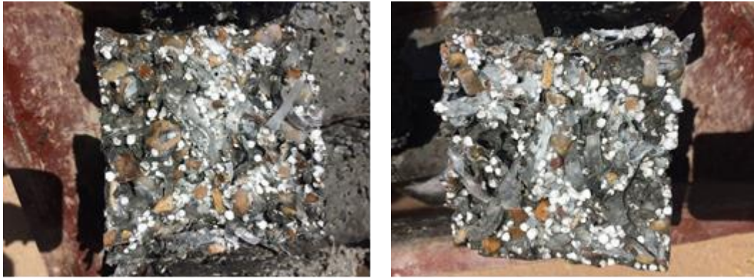
Figure 11. Photo of a cross section of prisms made of the mixes contain WPFs and Polystyrene and failed in flexure.
