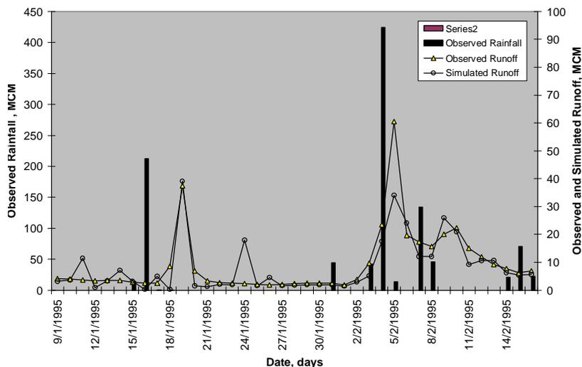
**Fig.(7): Observed and Simulated Runoff and Observed Rainfall for LVGFM Model (Verification Period), with a system memory ( $t=17$  days).**
