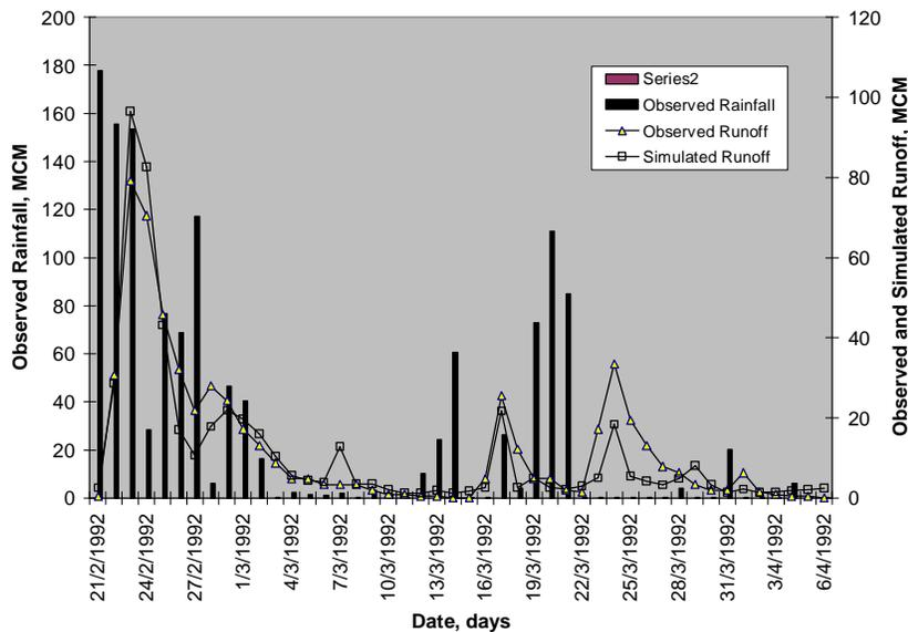
**Fig.(6): Observed and Simulated Runoff and Observed Rainfall for LVGFM Model (Calibration Period) with a System Memory ( $t=17$  days).**
