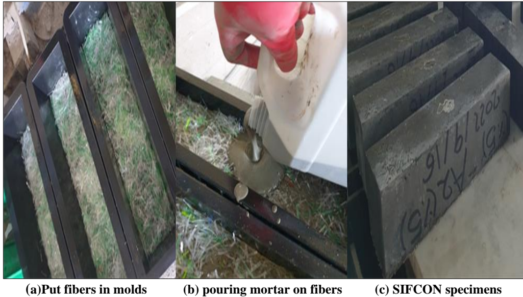
Fig .3 (a) ,(b) , and (c) Casting of SIFCON Mixtures
