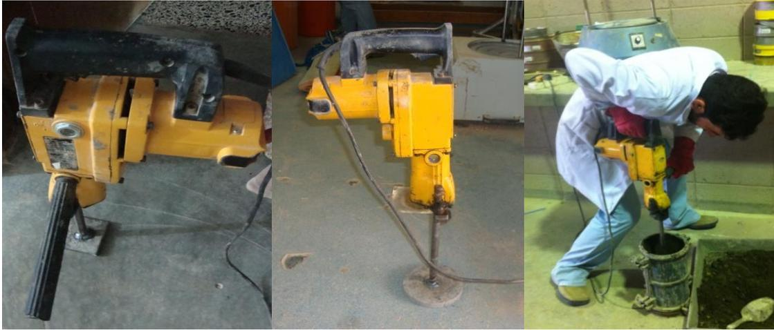
Fig (1): Vibrating Compaction Hammer with tamping plate
