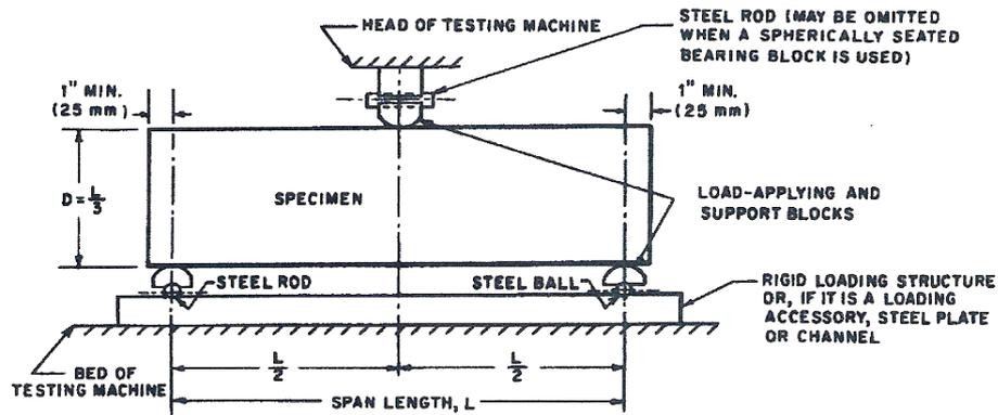
Fig(2):Diagrammatic View of a Suitable Apparatus for Flexure Test of Concrete by Center-Point Loading Method.
