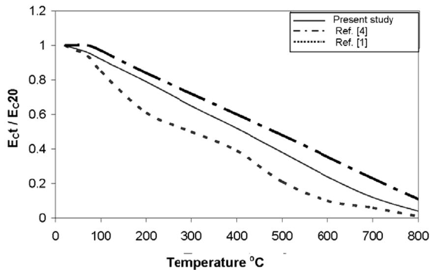
*Figure 2. Variation of modulus of elasticity with temperature rise.*
