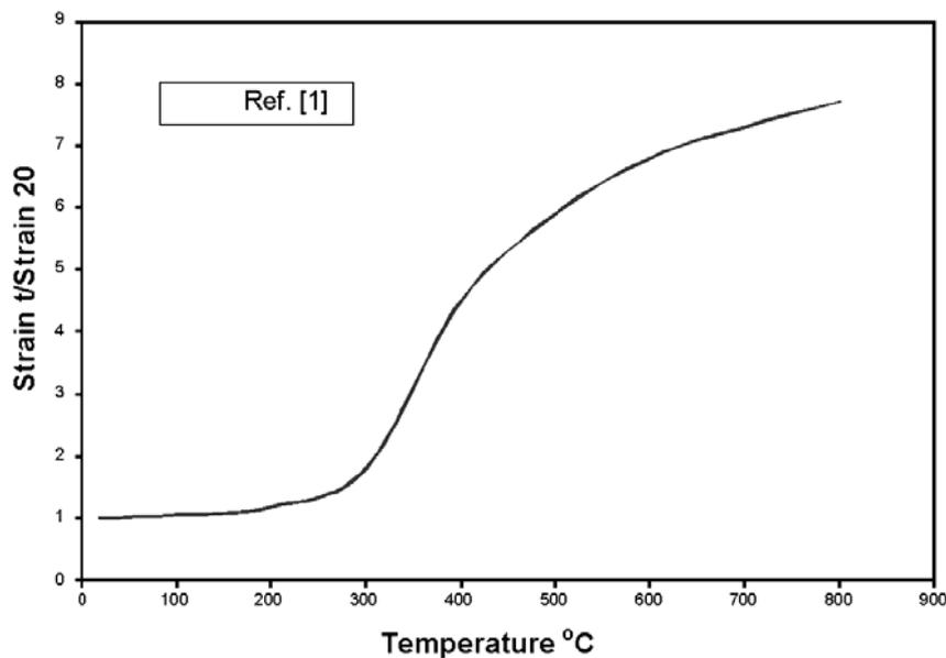
Figure 4. Variation of Strain with Temperature Rise.
