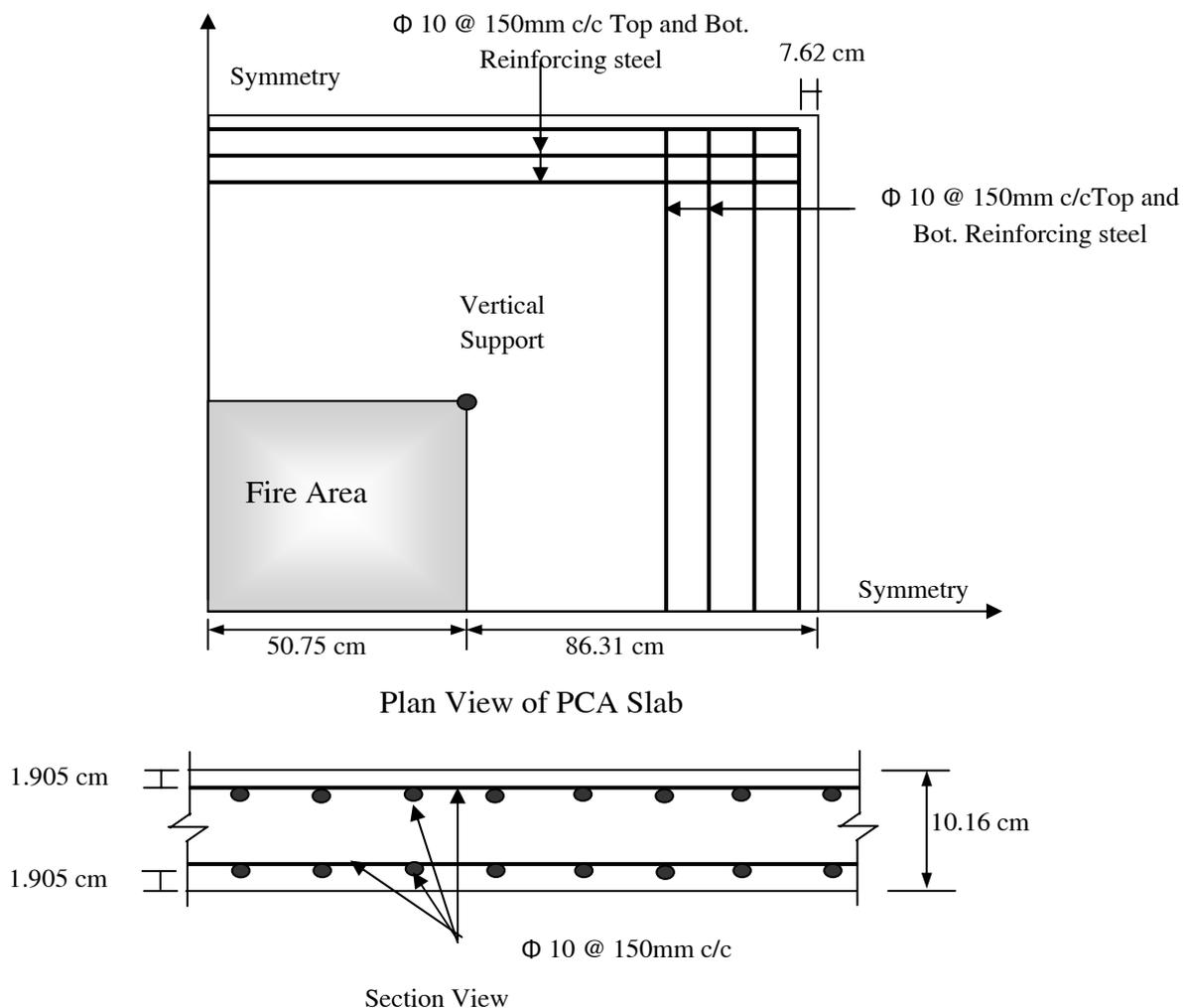
**Figure 10. The slab analysed by Brost and Peeters.**
