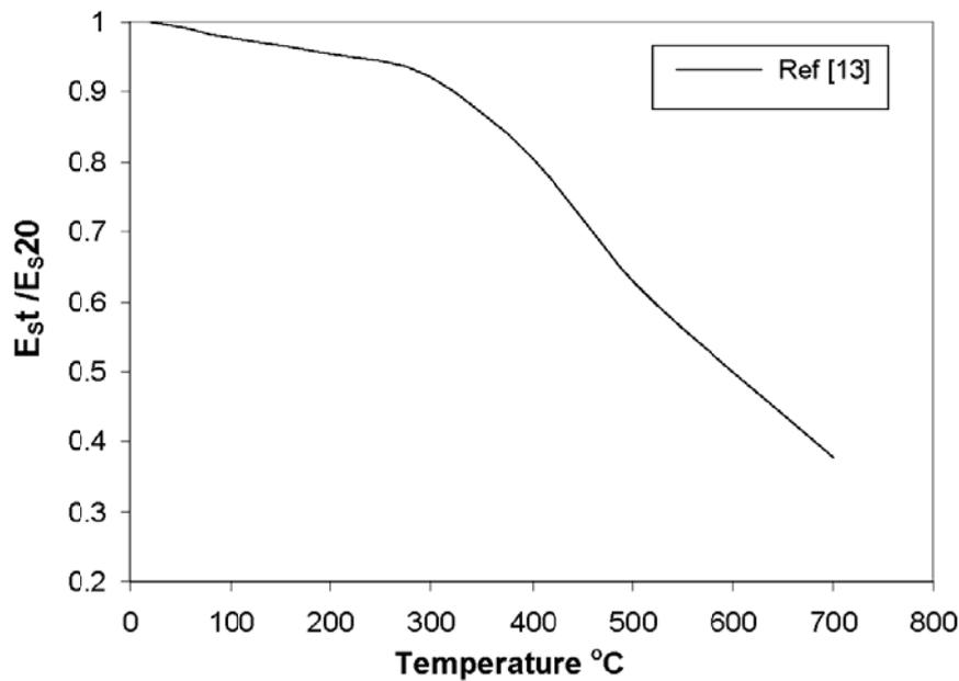
Figure 5. Variation of steel modulus with temperature rise.
