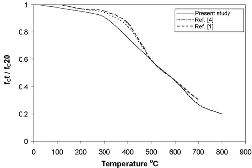
*Figure 1. Variation of concrete compressive strength with temperature rise.*
