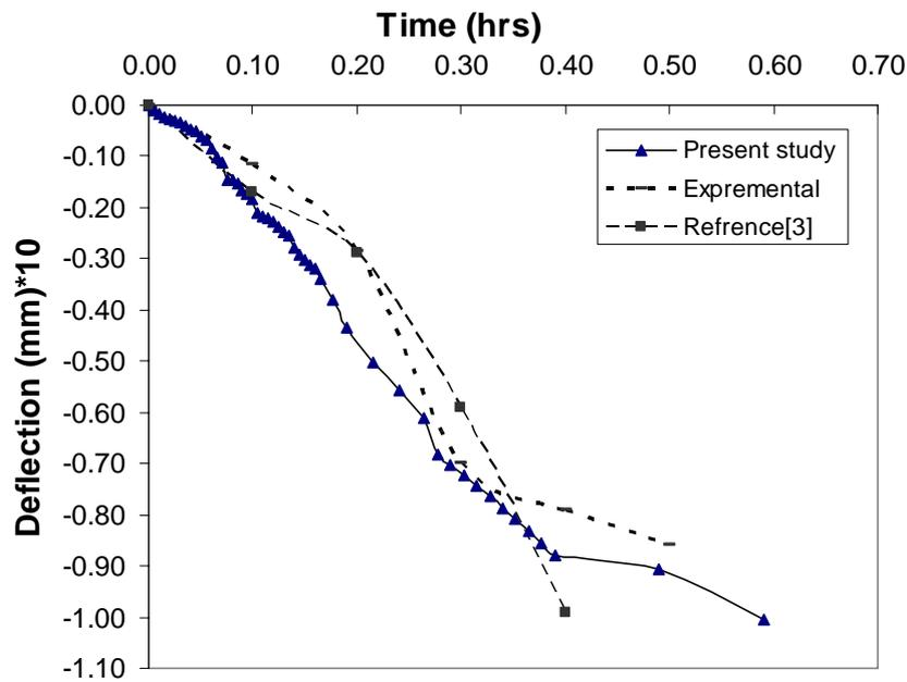
Figure 11. Experimental and calculated time-central deflection of reinforced concrete slab.
