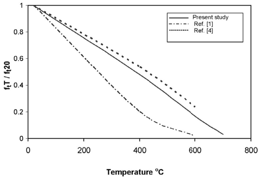
Figure 3. Variation of concrete tensile strength with temperature rise.
