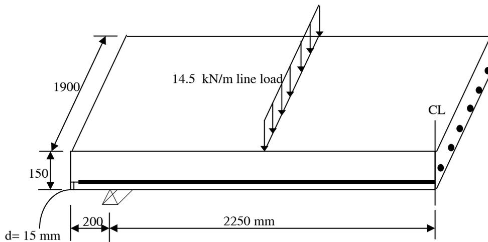
**Figure 8. The slab analysed by Brost and Peeters.**
