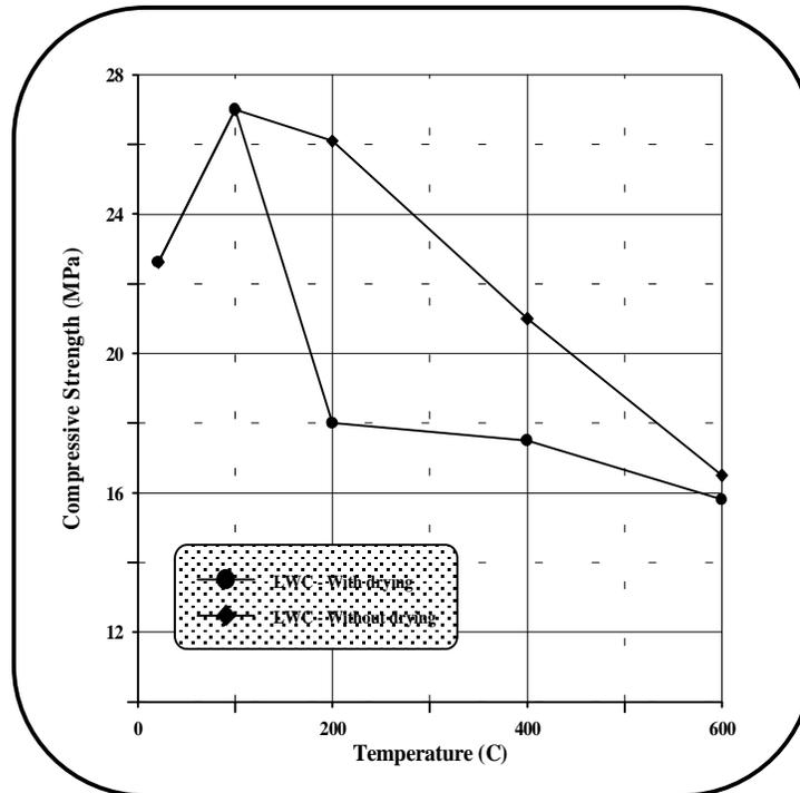
**Fig. (4 ) Effect of moisture content on Compressive strength-temperature relationships of SLWC at 28 day**
