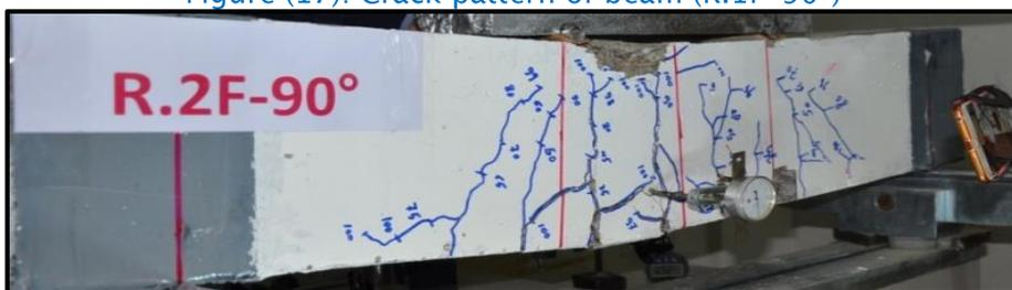
Figure (18): Crack pattern of beam (R.2F-90°)
