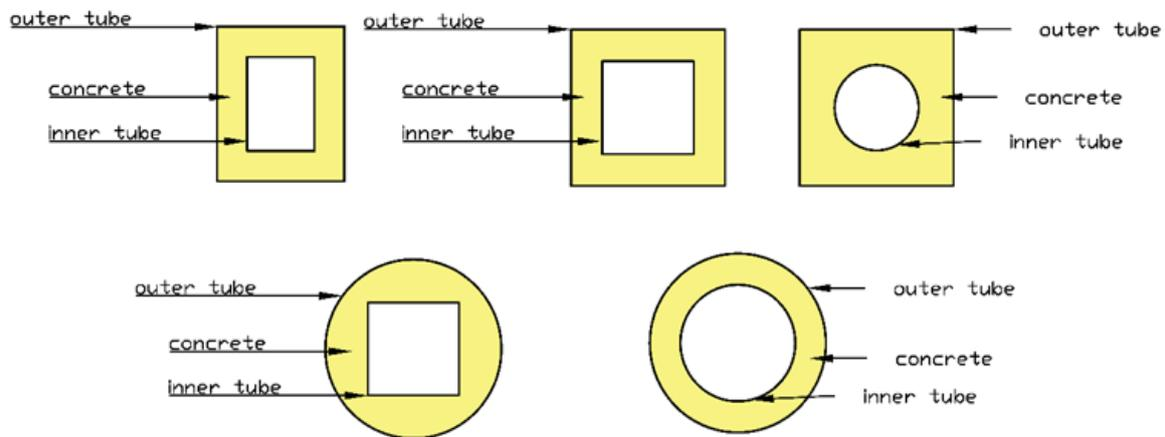
**Figure 1: Configurations of CFDST Column Cross Section**
