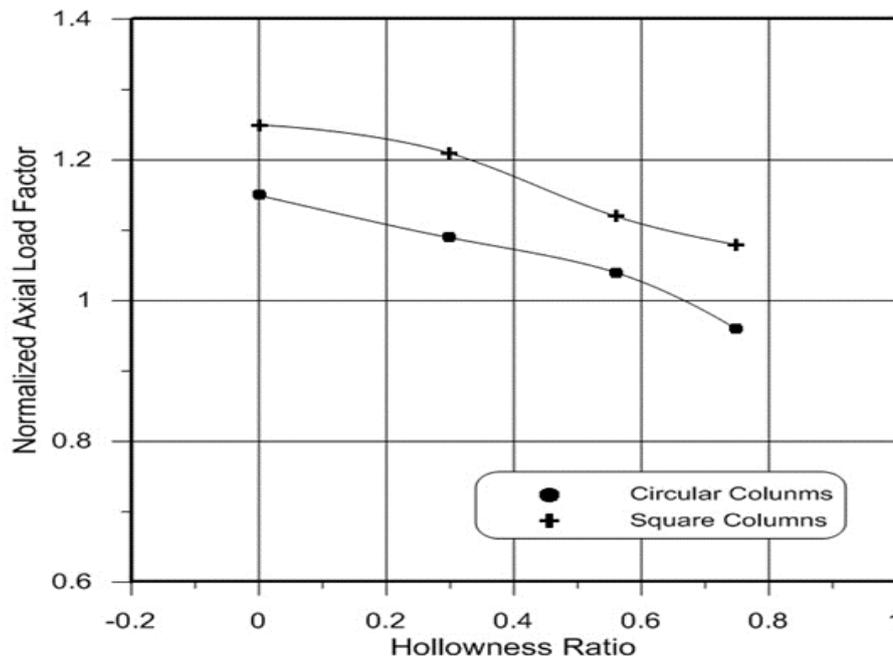
**Figure 9: Variation of Normalized Axial Load Factor with the Hollowness Ratio of Tested HSCFDST Specimens**
