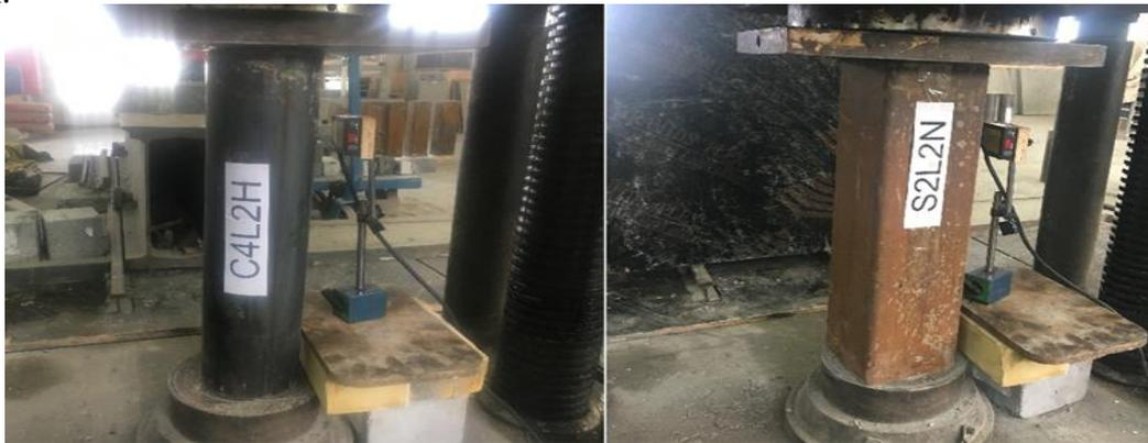
**Figure 4: Column Specimens Test Setup**
