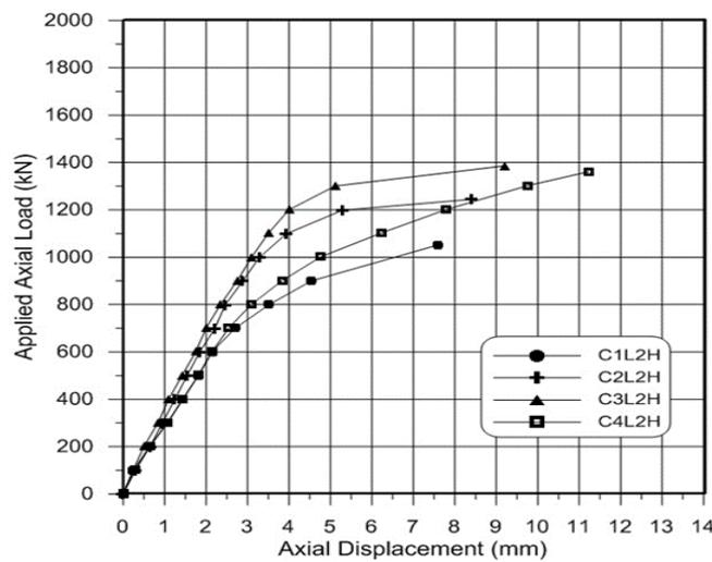
**Figure 7: Applied Axial Load - Axial Displacement Relationships for Tested HSCFDST Circular Specimens**
