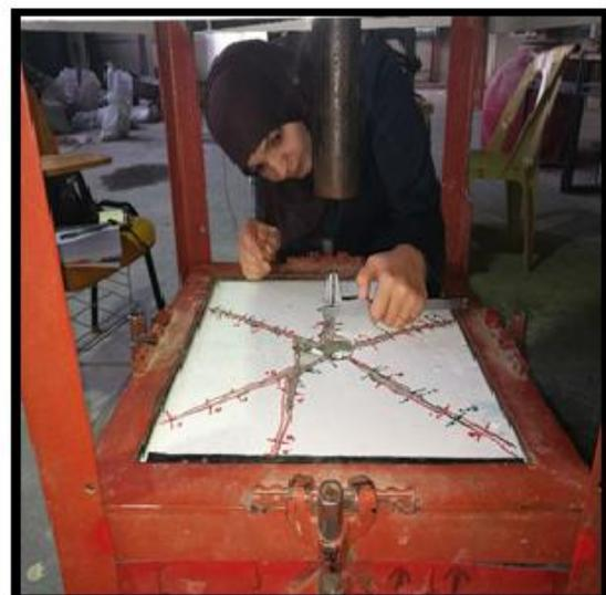
**b) Crack width measuring by Vernier Caliper**
