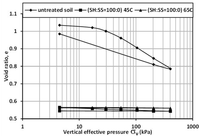
Fig. 5 Compression curves of untreated soil and soil-geopolymer (SH:SS=100:0)
