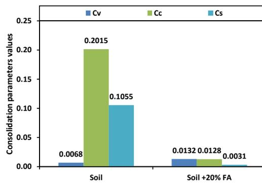
Fig. 4 Variation of compressibility parameters of soil+20% FA.
