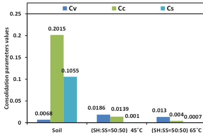
Fig. 8 Variation of consolidation parameters with (SH:SS=50:50) at different temperatures
