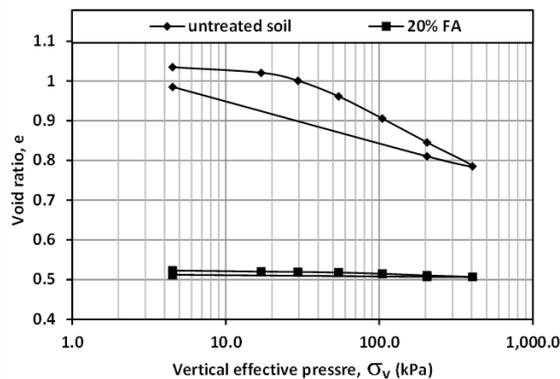
Fig. 3 Compression curves of untreated soil and soil+20% FA.
