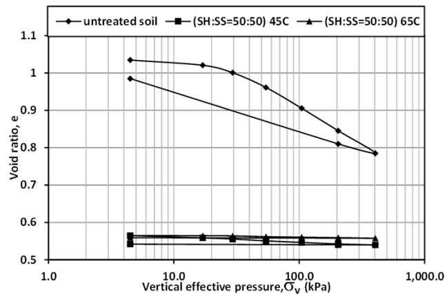
Fig. 7 Consolidation results of organic soil and soil- geopolymer blends using (SH:SS=50:50) at 8M
