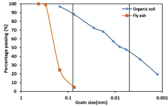
Fig. 1. Grain size distribution for the soil and fly ash
