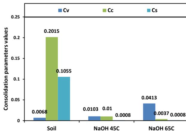
Fig. 6 Variation of the geopolymer-treated soil compressibility parameters (SH:SS=100:0).
