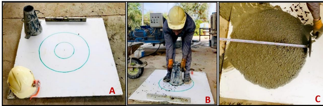
Fig. 3 [A] Slump wood Plate, [B] Raising cone test, [C] Measuring the diameter
