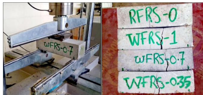
Figure 14 Flexural test machine and Specimens tested
