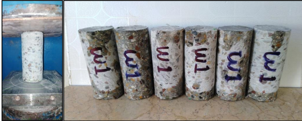
Fig. 11 Compressive testing of specimens
