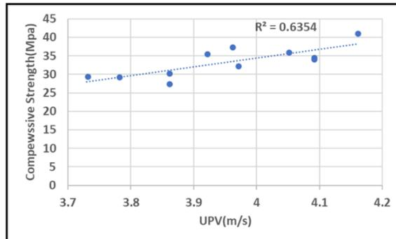
Figure 13 UPV and compressive strength relationship
