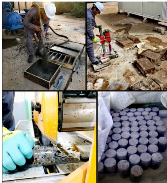
Fig. 2 Preparation processes of the core specimens
