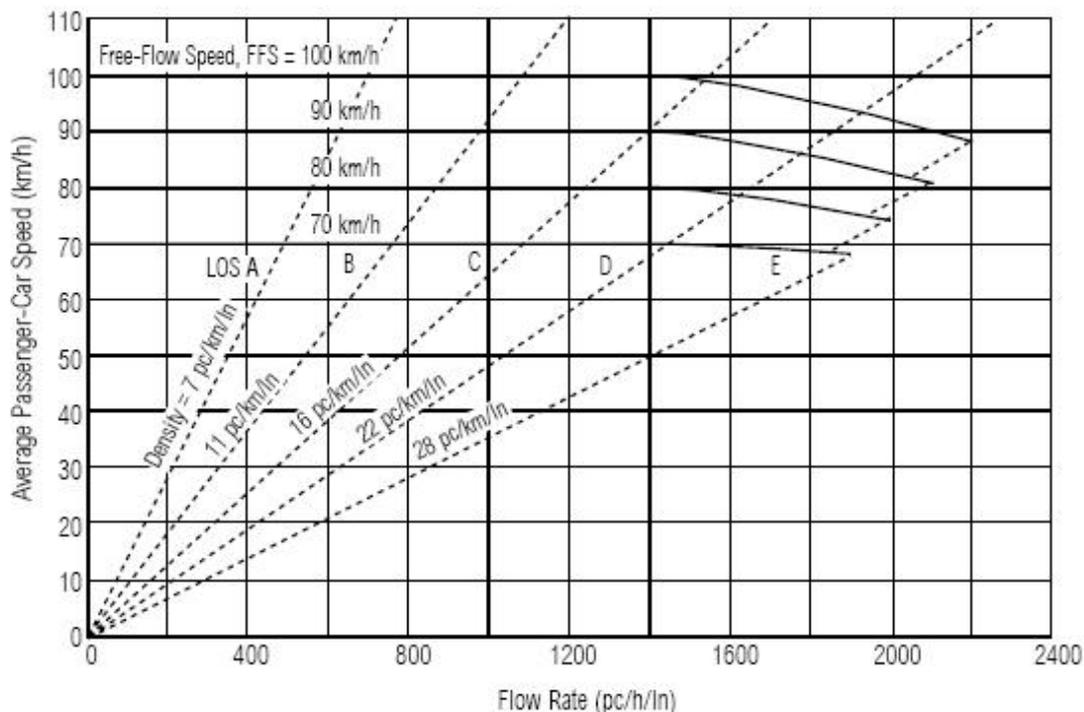
Figure 2. Speed-flow curves with los criteria for multilane highway.
