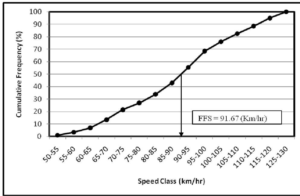
Figure 7. Free flow speed measurement in eastbound direction for multilane highway
