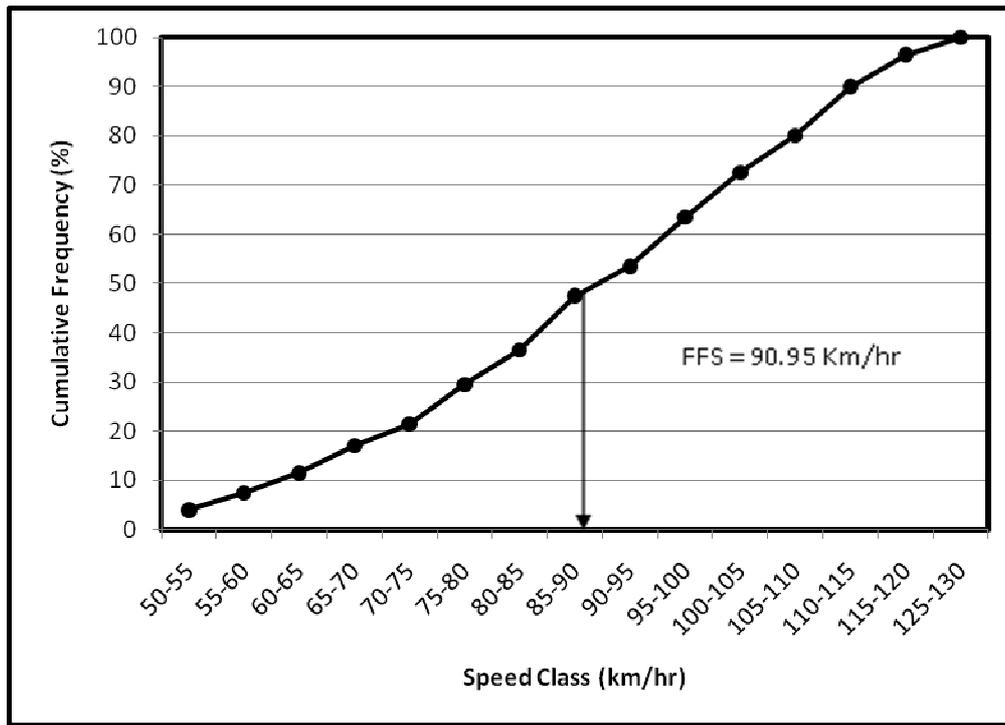
**Figure 6. Free flow speed measurement in westbound direction for multilane highway**
