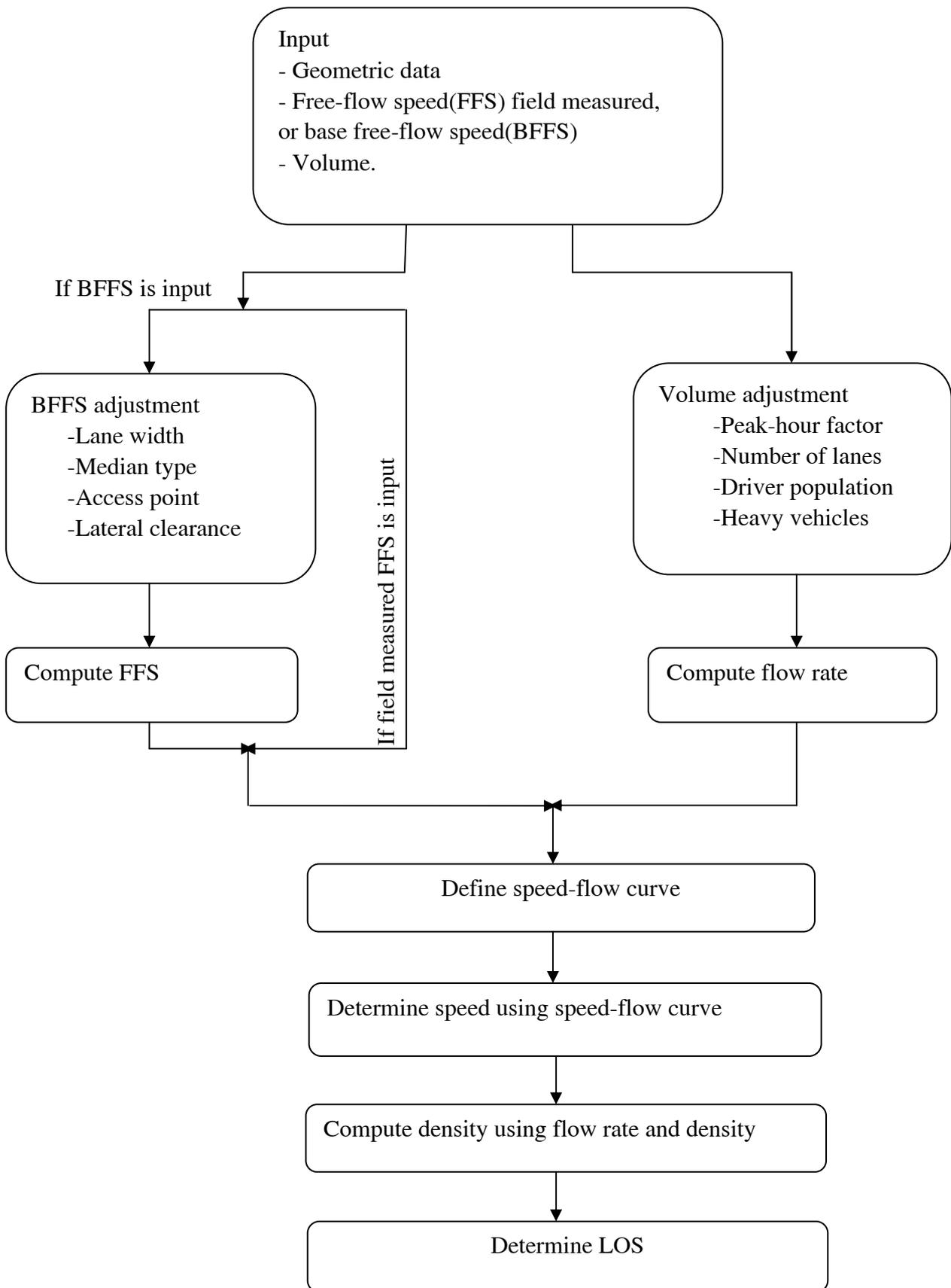
Figure1. Multilane highway methodology
