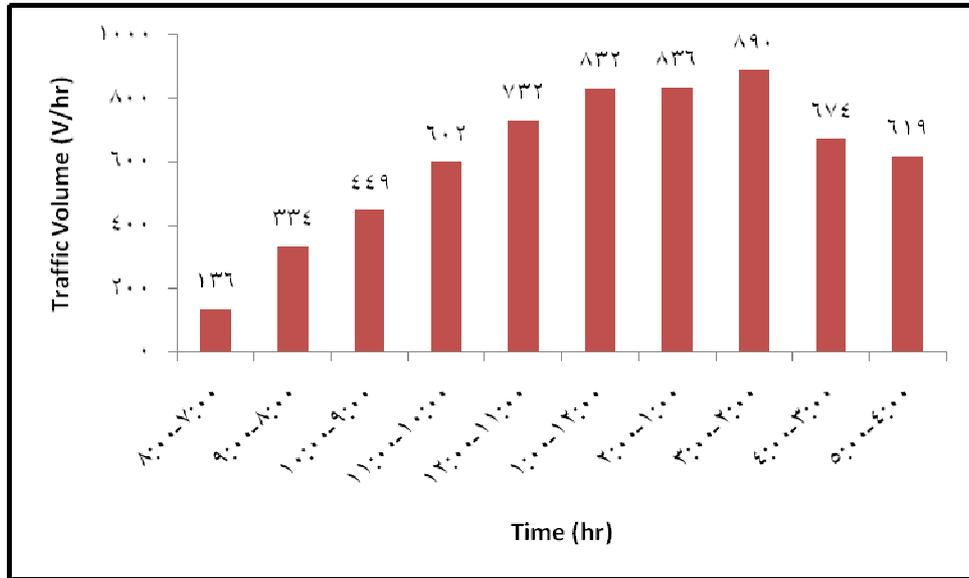
**Figure 5. Distribution of traffic volume during phv in eastbound direction for multilane highway**
