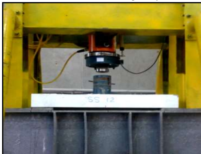
Plate (1): Slabs Setup on Hydraulic Testing Machine.
