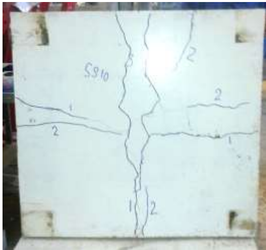
Figure(10): Numerical and Experimental Cracking Patterns of Thick Slab SS10 (Bottom Face).
