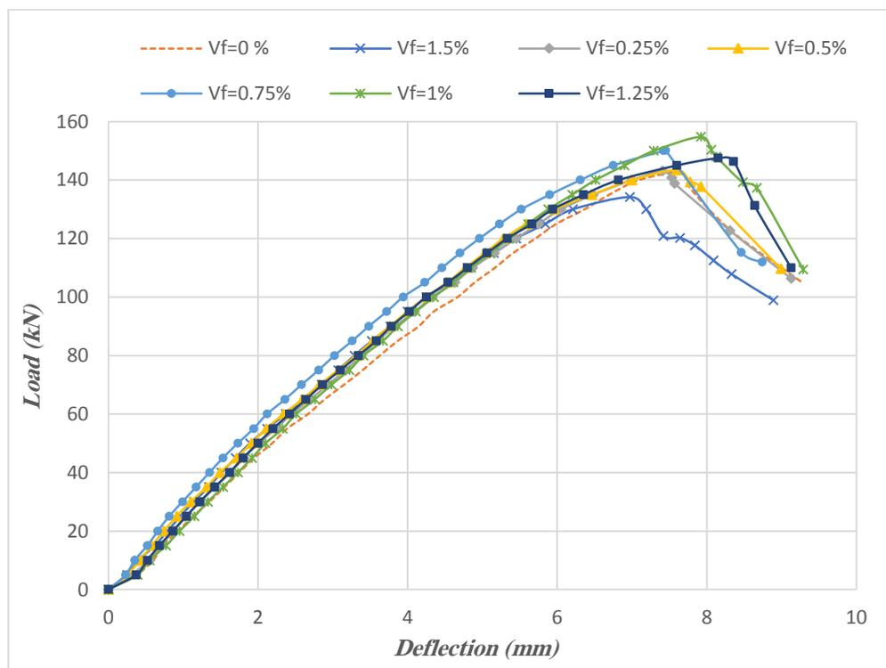
Figure 10. The relationship between load and deflection at mid span of all beams
