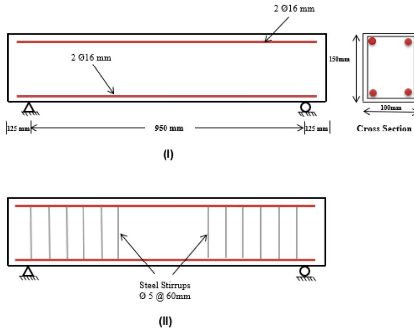
Figure 3. Beams reinforcement details
