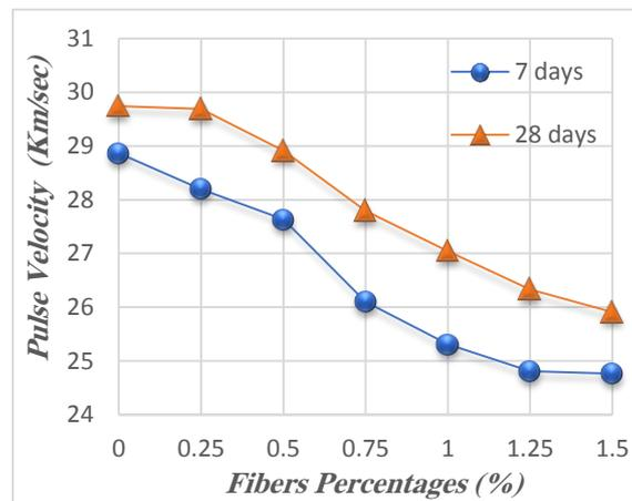
Figure 9. Relationship between the pulse velocity and fibers percentages
