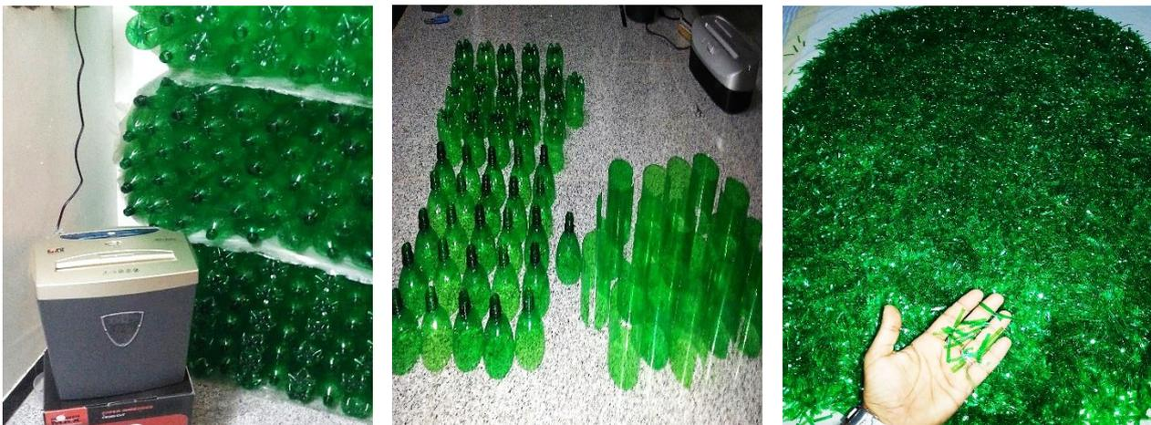
a) The paper shredder that was used for cutting the plastic bottles.
