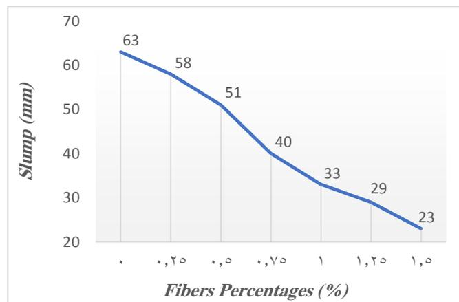
Figure 4. Effect of (PET) fibers on the workability
