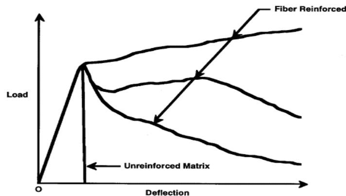
Figure 1. General load-deflection curves of Fiber Reinforced Concrete (FRC) and normal concrete<sup>[1]</sup>
