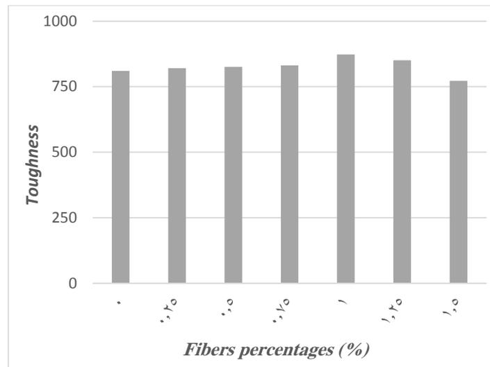
Figure 11. The area under load-deflection curve of all beams that were calculated by the AutoCAD and Excel software
