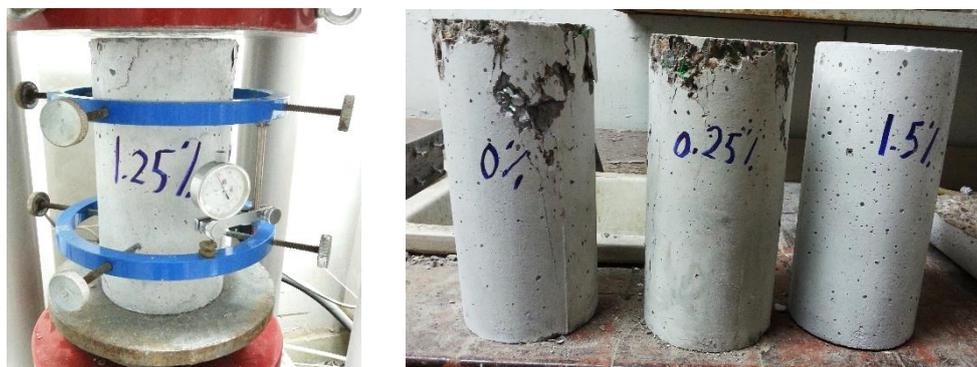
Figure 8. Static modulus of elasticity test
