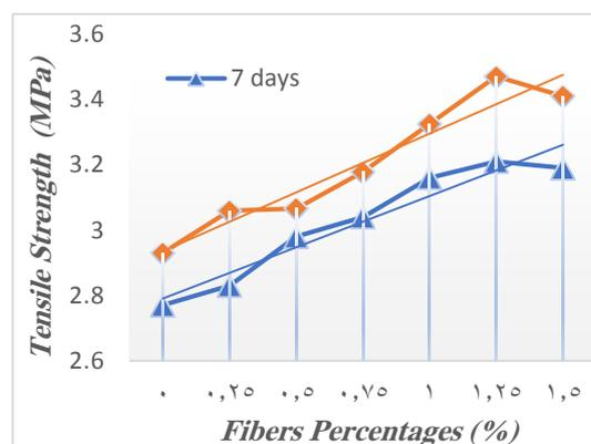
**Figure 5. Relationship between the splitting tensile strength and fibers percentages**
