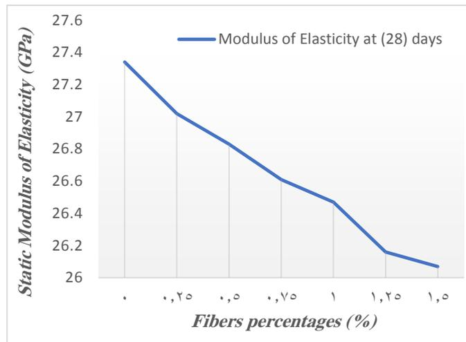
Figure (7) Relationship between the modulus of elasticity and fibers percentage
