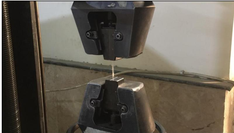
Fig. 3 The tensile strength test of PET fiber.
