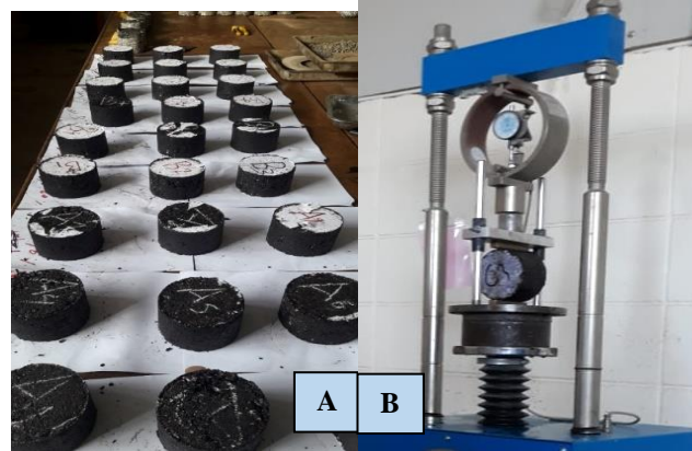
Fig. 8 (A) HMA specimens, (B) Indirect tensile strength (ITS) device
