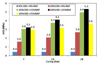
Fig. 7 UCS results for mixtures of 20% CKD with different RAP contents cured at different periods
