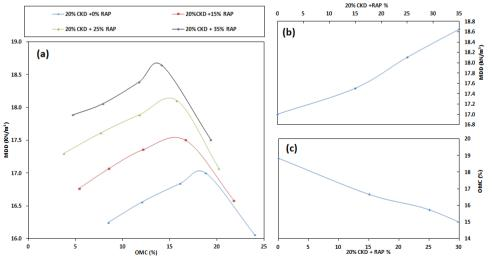
Fig. 3 Effect of CKD-RAP content on the compaction behavior of soil (a) compaction curves, (b) variation of MDD with CKD-RAP, (c) variation of OMC with CKD-RAP
