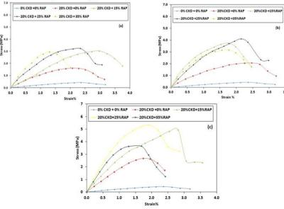
Fig. 6 Stress-strain of CKD-RAP mixture treated soil for varying curing periods: (a)7days (b)14days (c)28 days
