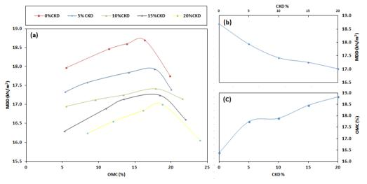
Fig. 2 Effect of CKD content on the compaction behavior of soil (a) compaction curves, (b) variation of MDD with CKD, (c) variation of OMC with CKD
