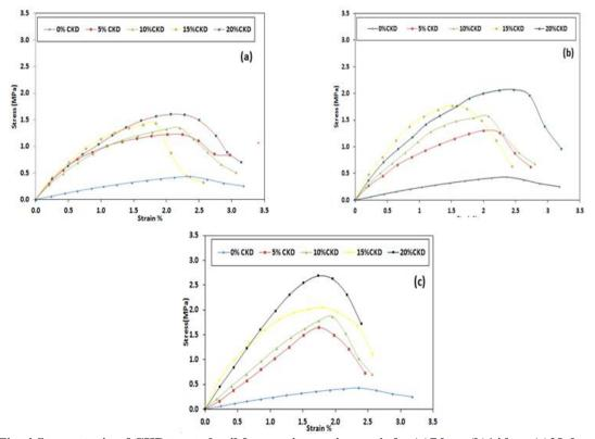
Fig. 4 Stress-strain of CKD treated soil for varying curing periods: (a)7days (b)14days (c)28 days
