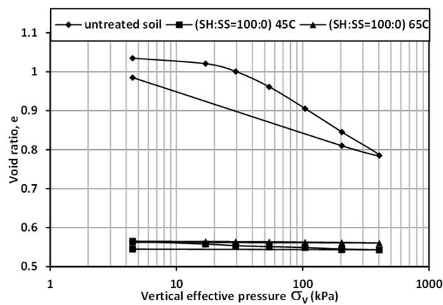
Fig. 5 Compression curves of untreated soil and soil-geopolymer (SH:SS=100:0)
