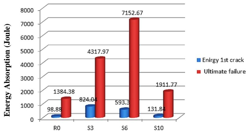
**Fig. 4 Energy required to occurs first crack and ultimate failure.**
