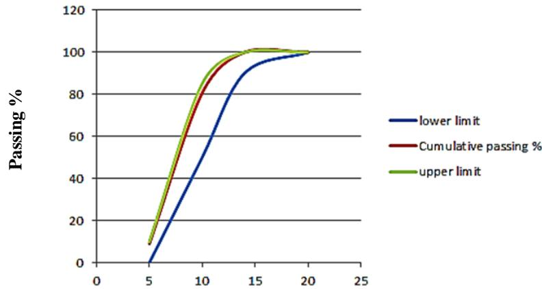
Fig. 2 Grading result of coarse aggregate (Mohammed, 2022).
