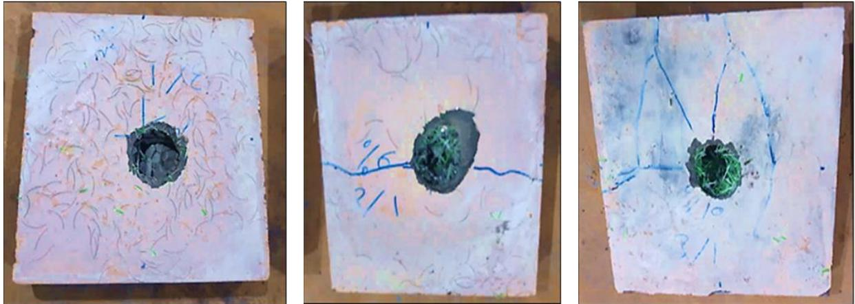
Fig. 5 Upper surface of impact resistance test of samples.
