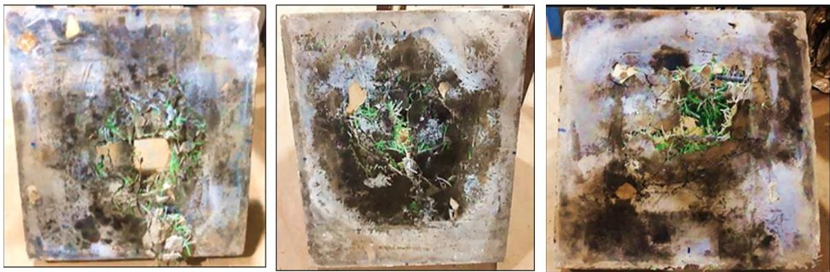
Fig. 6 Lower surface patterns of failure in concrete slabs.
