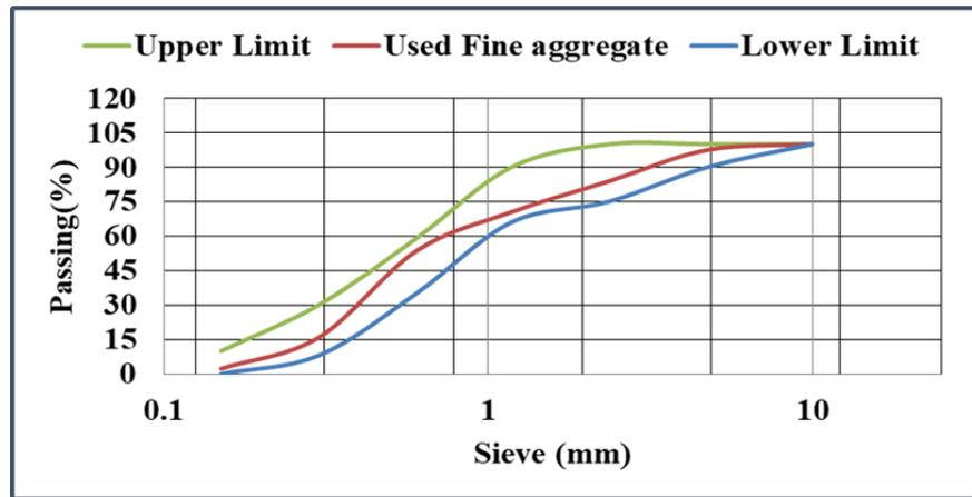
**Fig. 1 Grading result of fine aggregate (Mohammed, 2022).**
