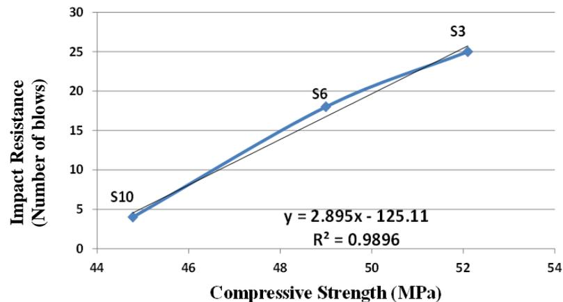
Fig. 7 Relationships between compressive strength and impact resistance at 70 day age for all concrete slabs.
