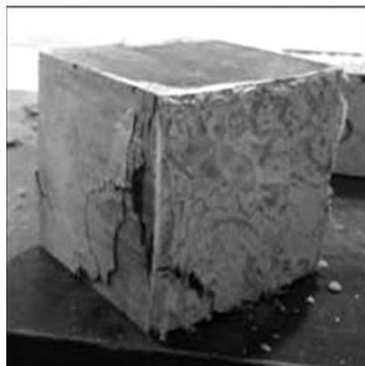
**Fig. 4 Failure form of SIFCON specimen**
