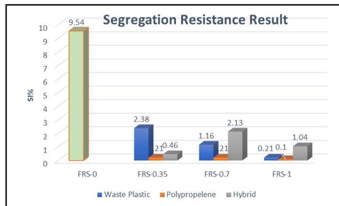
Fig. 6 Effect of fiber on the segregation resistance
