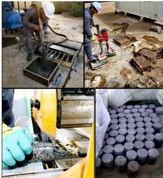
Fig. 2 Preparation processes of the core specimens
