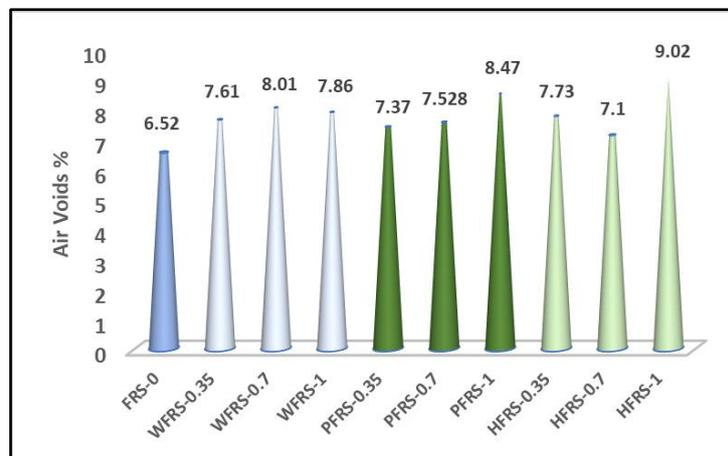
**Fig. 7 Effect of fiber on the Air Voids.**
