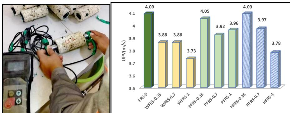
Fig. 10 Ultrasonic pulse velocity test and results
