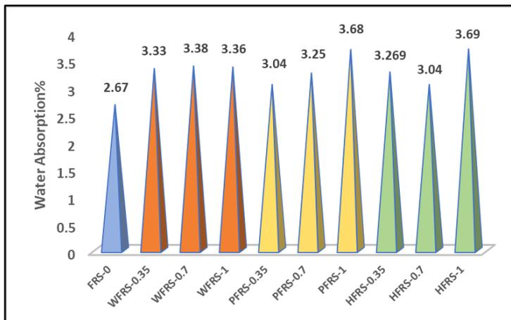
Fig. 8 Effect of fibers on the water Absorption
