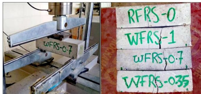
Figure 14 Flexural test machine and Specimens tested
