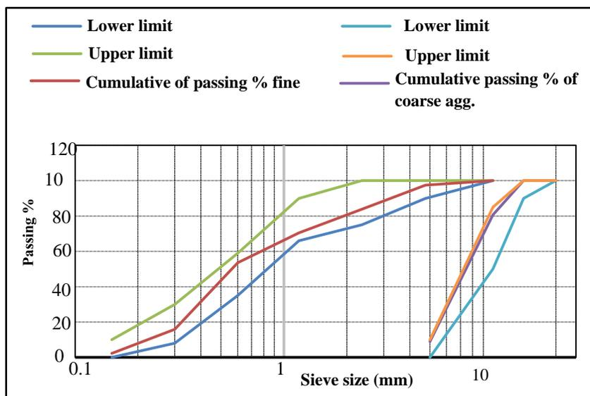
Fig. 2 Grading curves of fine and coarse aggregates
