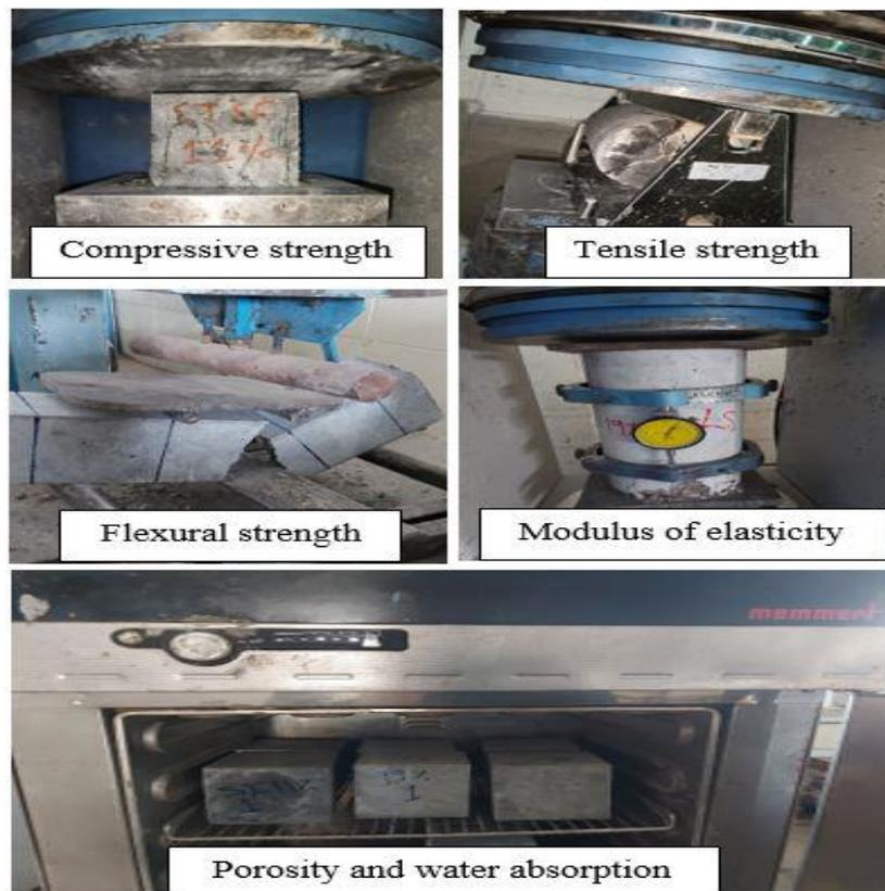
Fig. 5 Mechanical and related durability properties' tests
