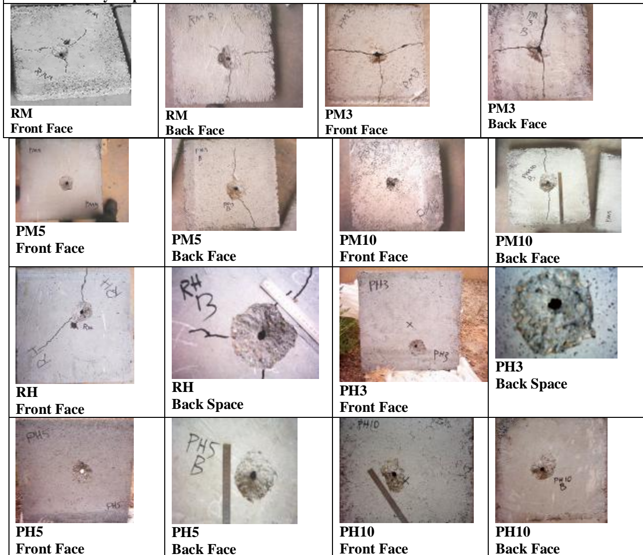
Plate(5): The Mode of Failure of Slabs under High Velocity Impact
