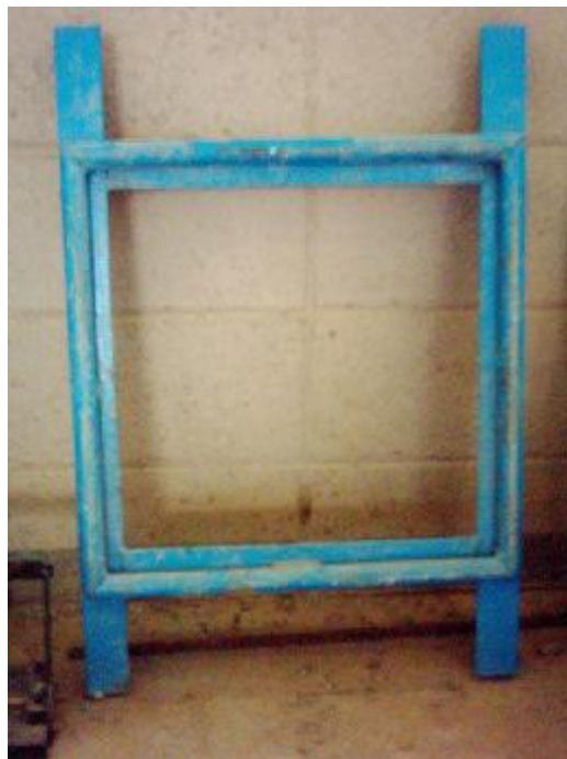
Plate(1):a-Test rig Used for Low Velocity Impact Test b-Frame Used for Supporting Impact Slabs
