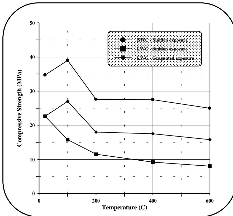
**Fig. (2 ) Compressive strength-temperature relationships of SLWC and NWC under high temperature at 28 day**
