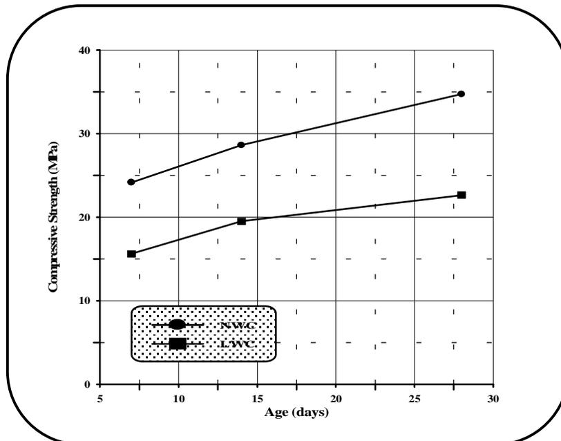
Fig. (1 )Development of compressive strength of SLWC and NWC
