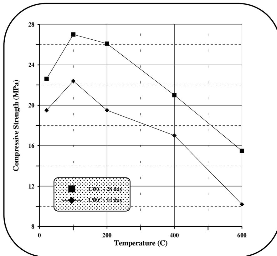
**Fig. (3 ) Compressive strength-temperature relationships of SLWC under high temperature**
