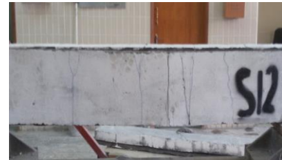
Figure 12.4: Cracks Pattern of Specimen SI2
