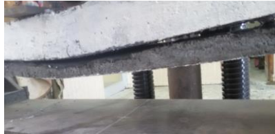
(a) Debonding failure
