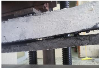
(a) Debonding failure
