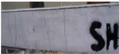
Figure 12.1: Cracks Pattern of Specimen SH1
