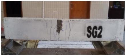
Figure 8.4: Cracks Pattern of Specimen SG2
