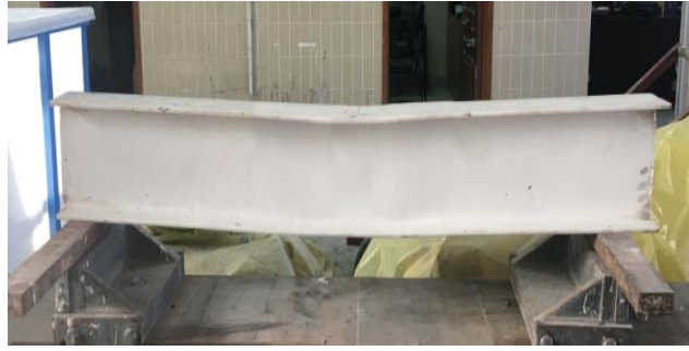
Figure 14. Failure Mode of specimen C0
