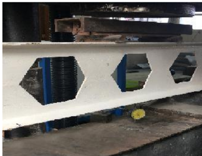
Figure (3): Test Set up of Castellated Beam
