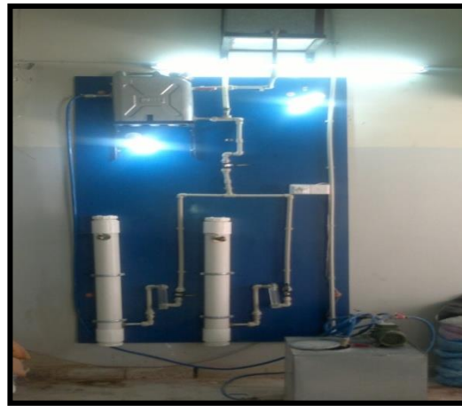
Fig.(4): The physical model (filter columns).
